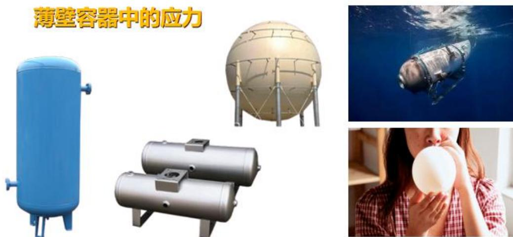
**轴向应力**  $\frac{\pi D^2}{4} \cdot p = \pi D \delta \cdot \sigma_a \quad \sigma_a = \frac{Dp}{4\delta}$
